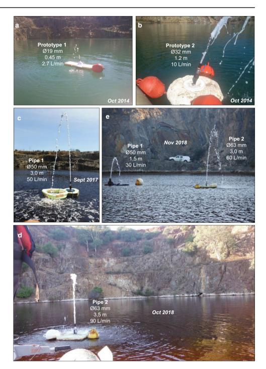
larger pipe (Pipe 2, 63 mm diameter and 65.5 m in length) was installed in June 2017 (Fig. 3b).
